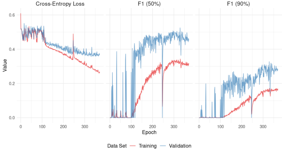
Figure 3: Loss and evaluation metrics during training for our segmentation model. It took about 100 epochs for the model to start learning. After 370 epochs, we decided to halt training as it appeared the model was starting to overfit. For deployment, we used the 305-epoch model.
